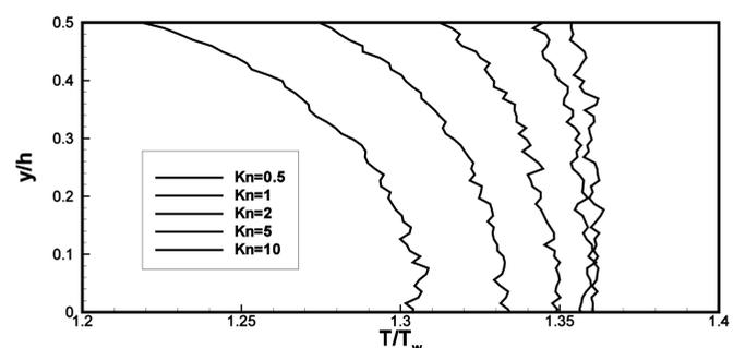
Fig.3- Rarefaction Effects on Temperature Profiles
