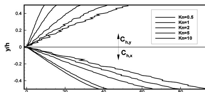
Fig.4- Rarefaction Effects on Heat Flux Profiles
