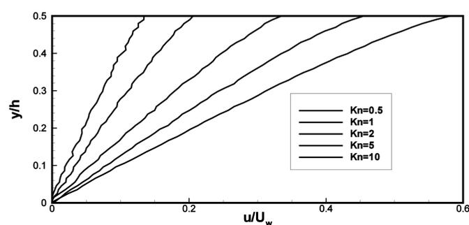
Fig.2- Rarefaction Effects on Velocity Profiles
