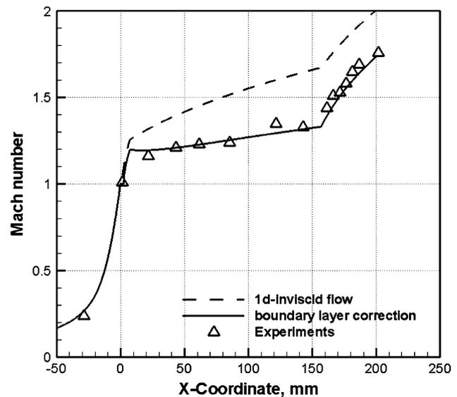
**Fig. 7** Mach number plot along the first nozzle
