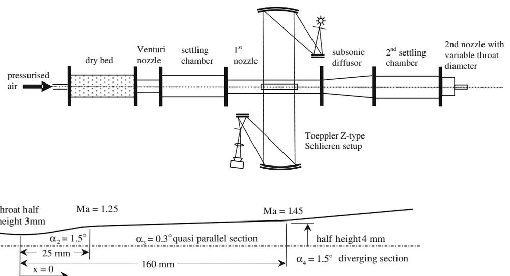
**Fig. 5** Sketch of the nozzle contour
