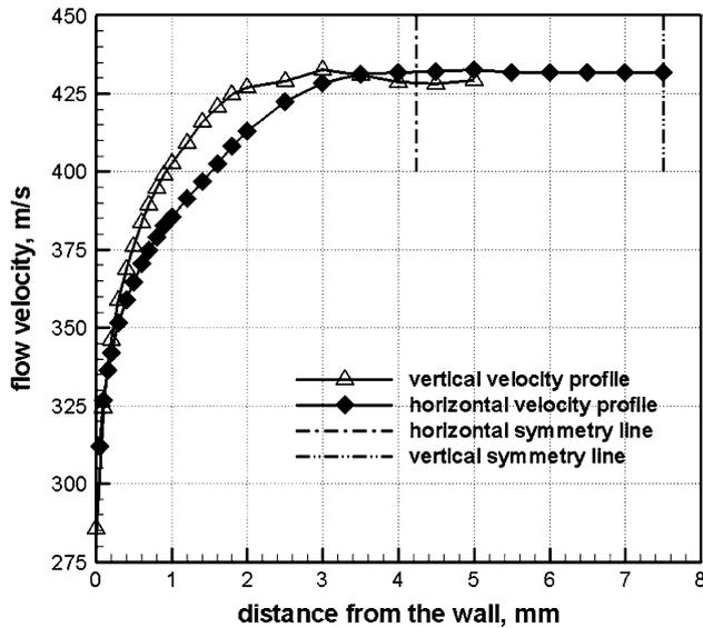
**Fig. 8** Horizontal and vertical boundary layer profile
