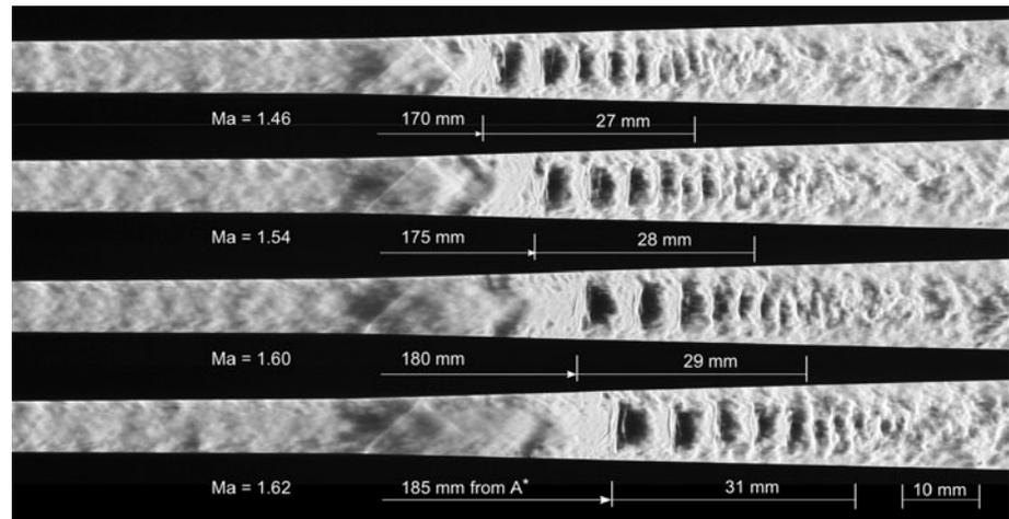
different back pressure. As the Mach number changes from 1.46 to 1.62 the shock train becomes longer, and the turbulent mixing is much stronger. For the sake of correctness one must note that due to the relocation of the shock train the Reynolds number  $Re_\theta$  also changes.
